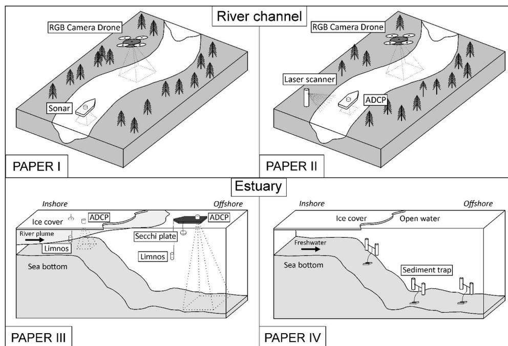
**Figure 6.** Schematic picture of field methods used in each paper. Methods are described more detail in the text and table 1. Papers I and II focus on river and papers III and IV on estuary environment.
