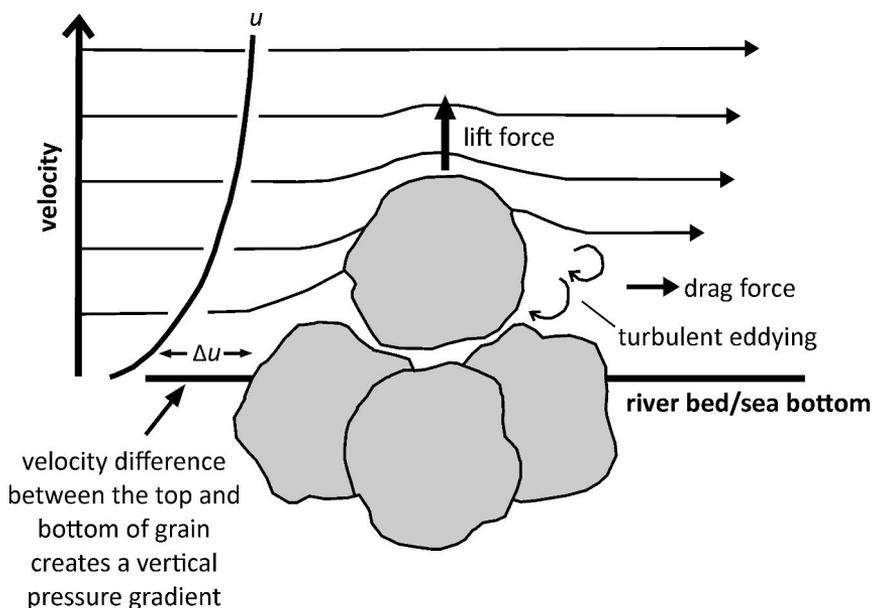
**Figure 2.** Forces acting on sediment particle entrainment. Drag and lift forces, associated with flow turbulence, entrain grains from the bottom. The vertical pressure gradient, caused by the difference in velocity ( $u$ ) between the top and bottom of a grain, induces lift force. In addition, entrainment depends on particle size and the extent to which the particle protrudes into the flow or is embedded against other grains. Modified from Knighton (1998) and Fryirs and Brierley (2013).
