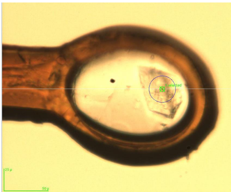
Figure 14. Dpr crystal (~40 \mu\text{m} size) corresponding to condition 9 that gave the best diffraction pattern and the 2.2 Å full dataset. The loop size is 100 \mu\text{m} .
