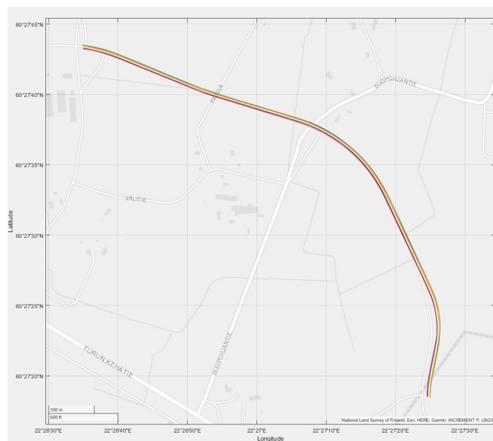
Figure 5.3: The absolute lateral error of GNSS for each drive of the first experiments. Each drive is separated by a line.
