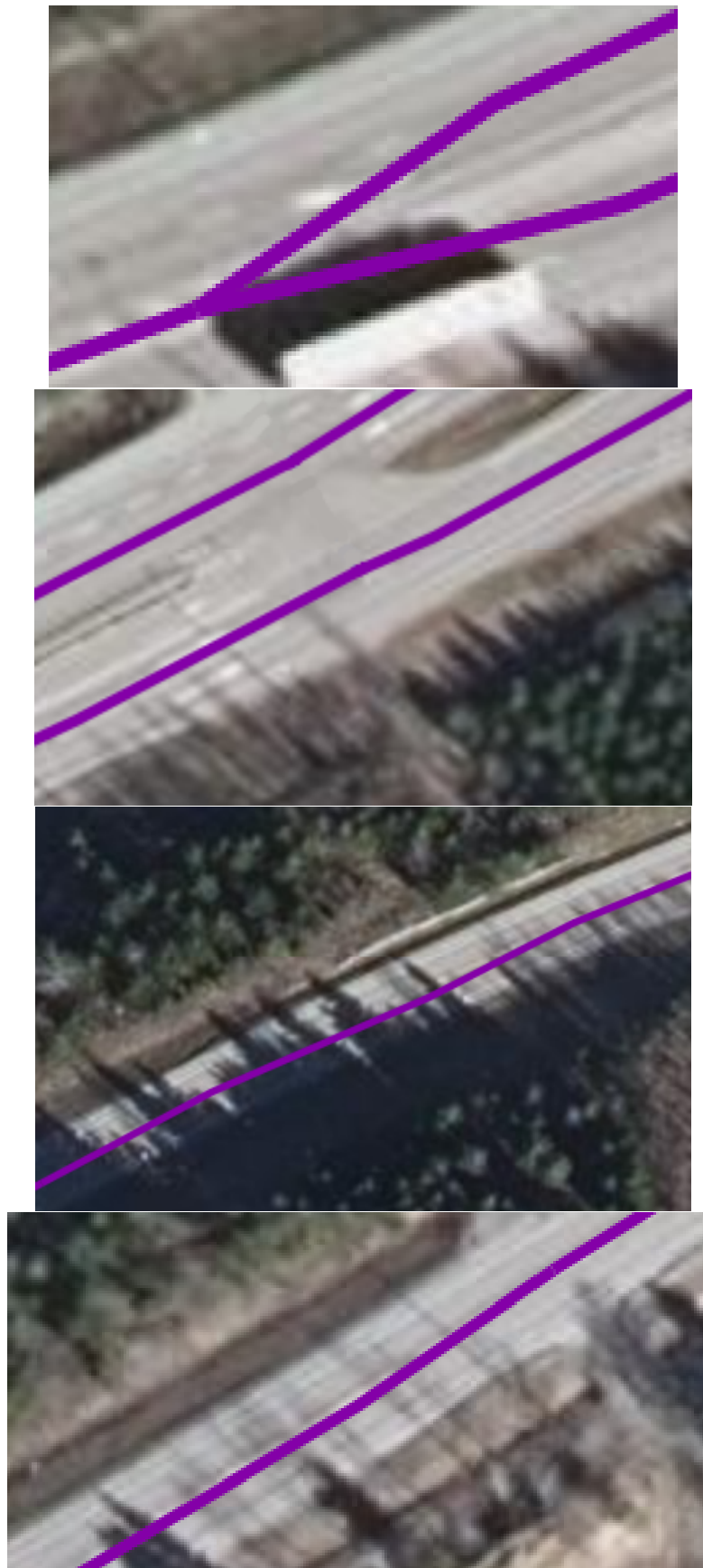
Figure 5.10: Road positions on the map that do not follow the center of the road.
