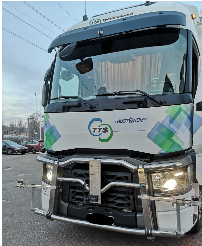
Figure 4.3: The truck and its LIDAR sensors used for the second experiment
