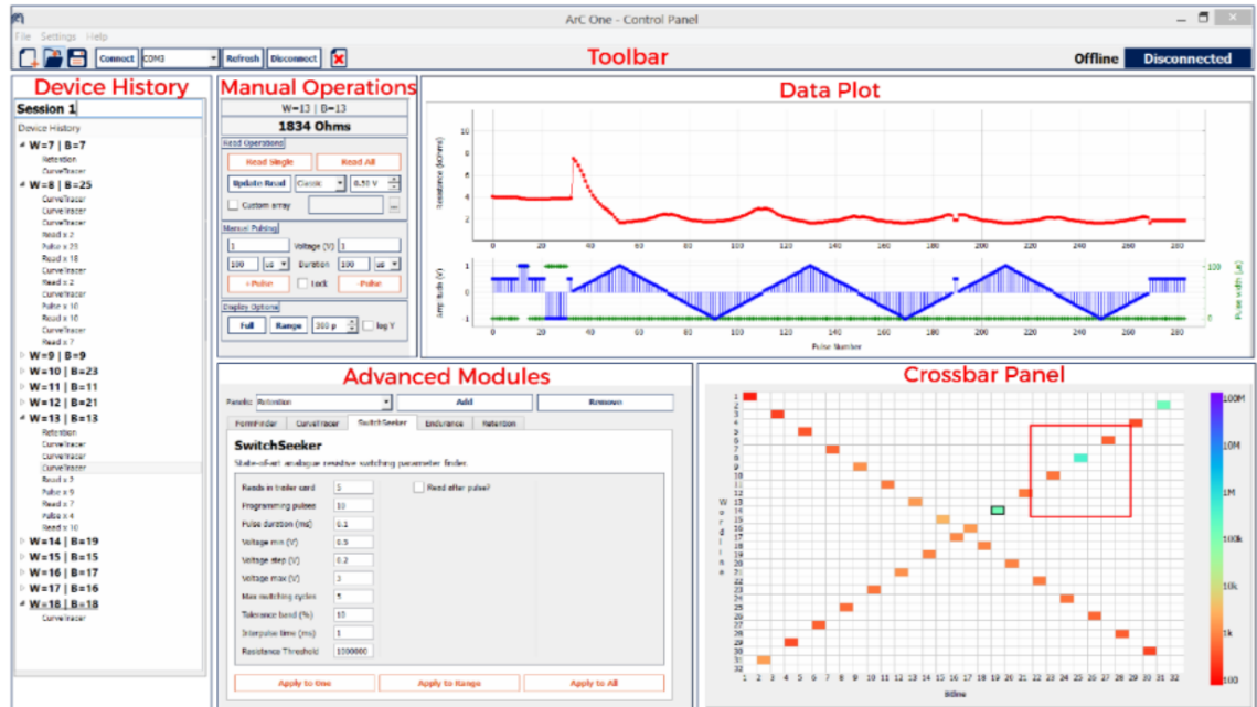
Figure 9. ArC ONE user interface and the functional panels: Device History, Manual Operations, Toolbar, Data Plot, Advanced Modules, and Crossbar Panel [35].
