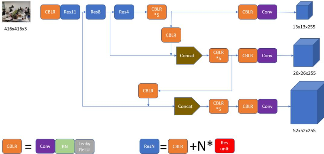
Figure 3-8 Neural Network Structure of YOLOV3
