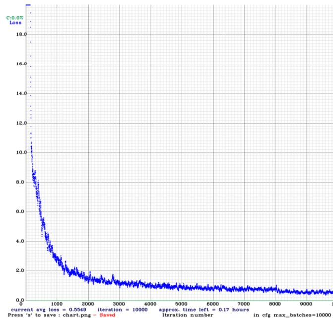
Figure 3-14 Training Process of YOLOV4
