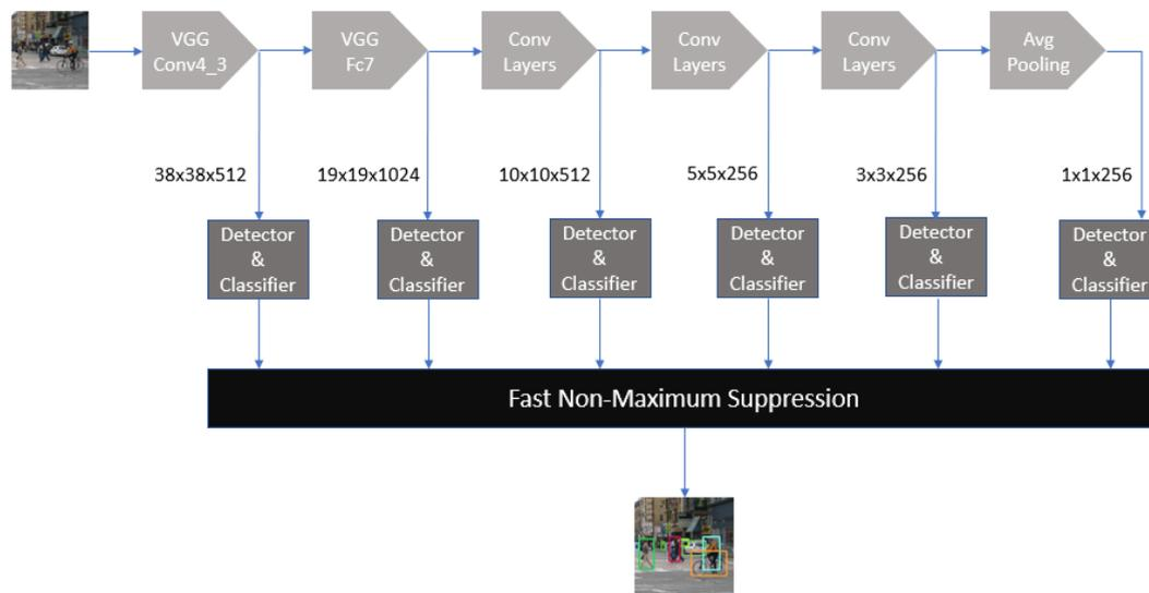
Figure 3-3 Neural Network Structure of SSD
