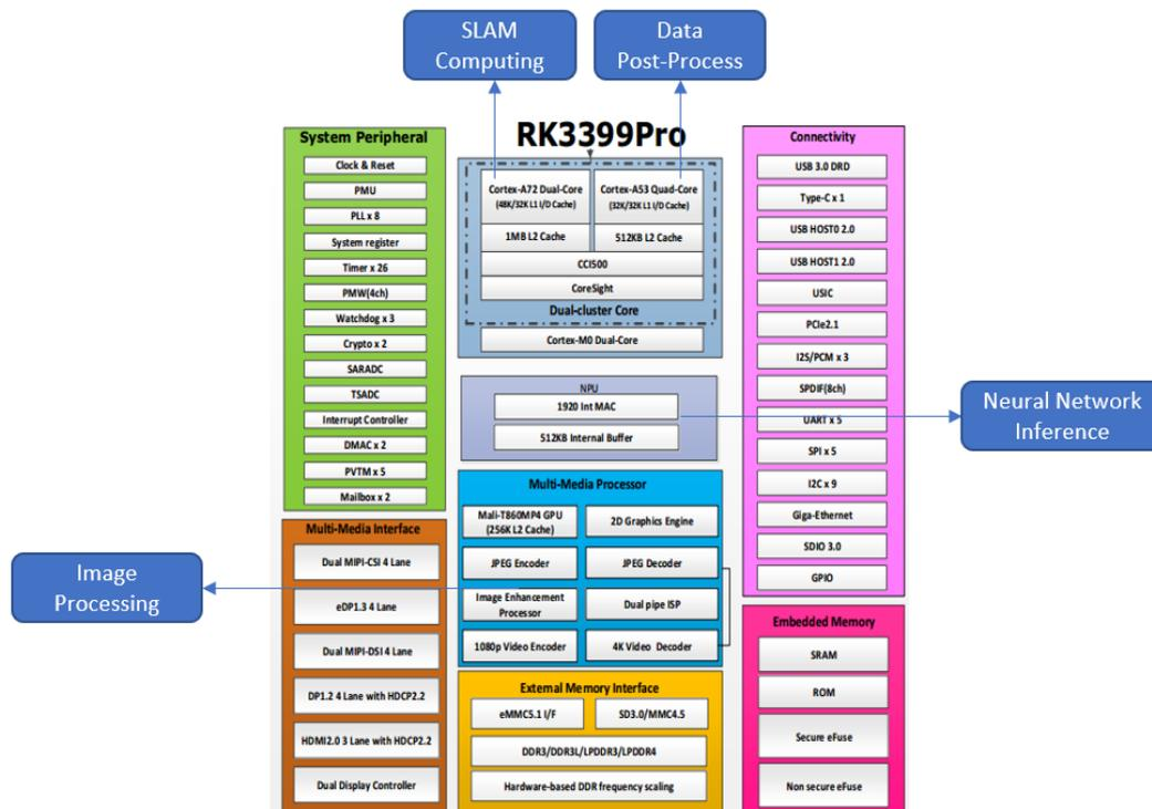
Figure 4-2 RK3399PRO Soc Architecture
