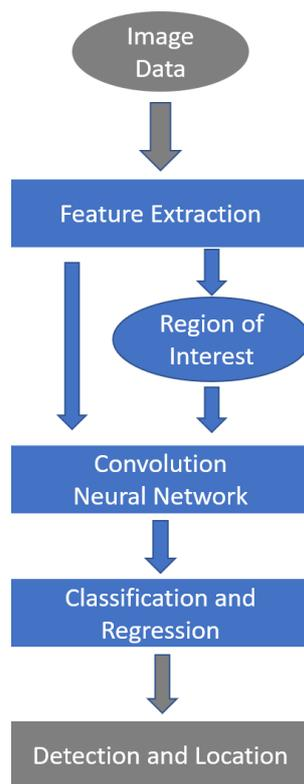
Figure 2-3 Main Idea of Object Detection based on Deep Learning
