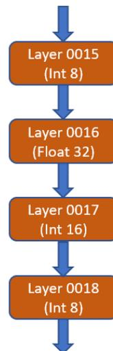
Figure 4-11 Mixed Precision Process
