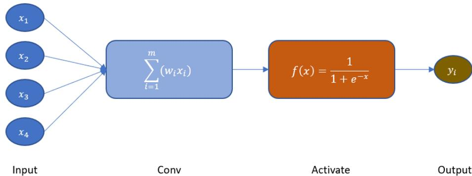
Figure 4-12 Activation Function Process
