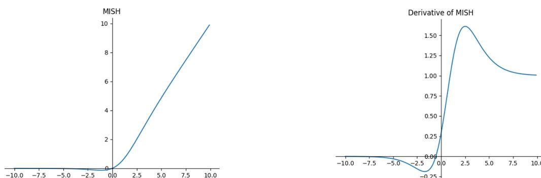
Figure 4-17 Mish Function Curve
