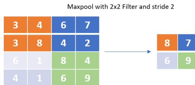
Figure 4-20 Max Pooling Process
