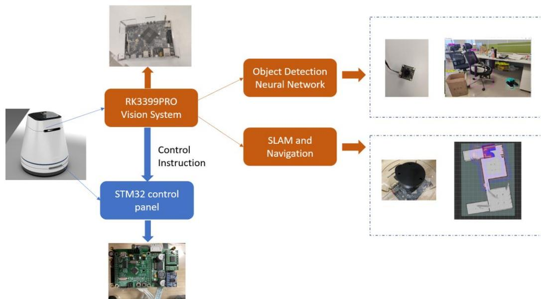
Figure 2-4 Whole Vision System Architecture
