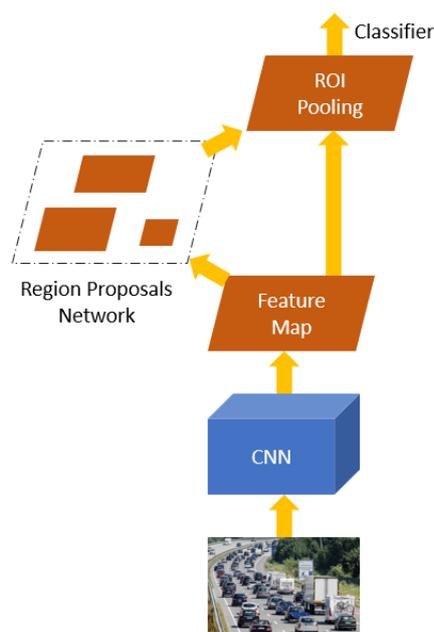
Figure 3-2 Neural Network Structure of Faster-RCNN
