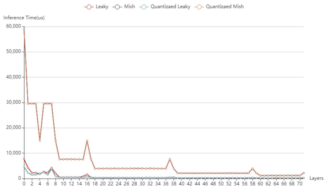
Figure 4-18 Inference Time of Leaky ReLU and Mish Layers on RK3399PRO
