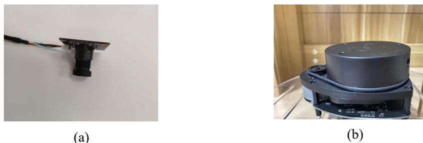
Figure 2-1 Sensors of Vision System (a)Monocular camera (b)2D LiDAR
