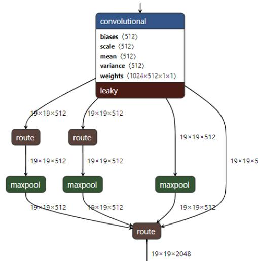
Figure 3-13 Structure of SPP
