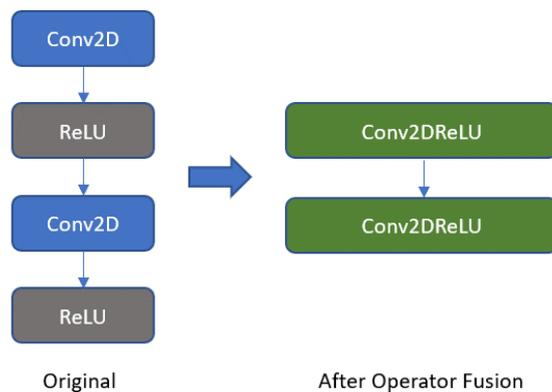
Figure 4-19 Operator Fusion of ReLU
