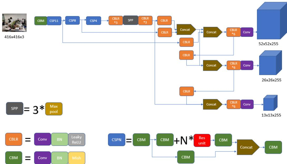
Figure 3-12 Neural Network Structure of YOLOV4
