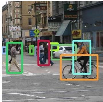
Figure 3-4 Inference Result of SSD on RK3399PRO
