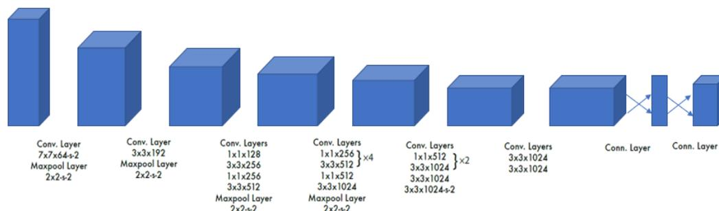
Figure 3-5 Neural Network Structure of YOLO
