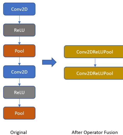
Figure 4-22 Operator Fusion of Pooling
