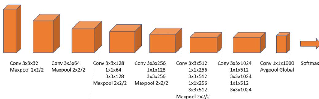
Figure 3-6 Neural Network Structure of YOLOV2
