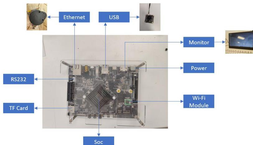
Figure 4-3 Development Board Connection Diagram
