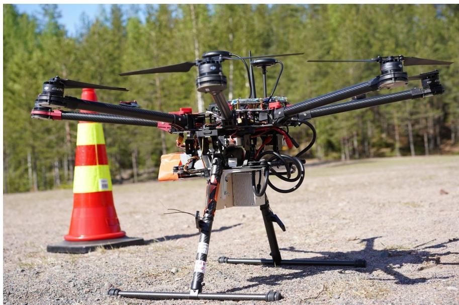
Figure 4.2: DJI S1000 equipped with solid state LIDAR sensor
