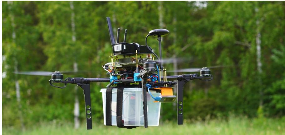
Figure 4.8: Drone connected to the 5G network through USB tethering
