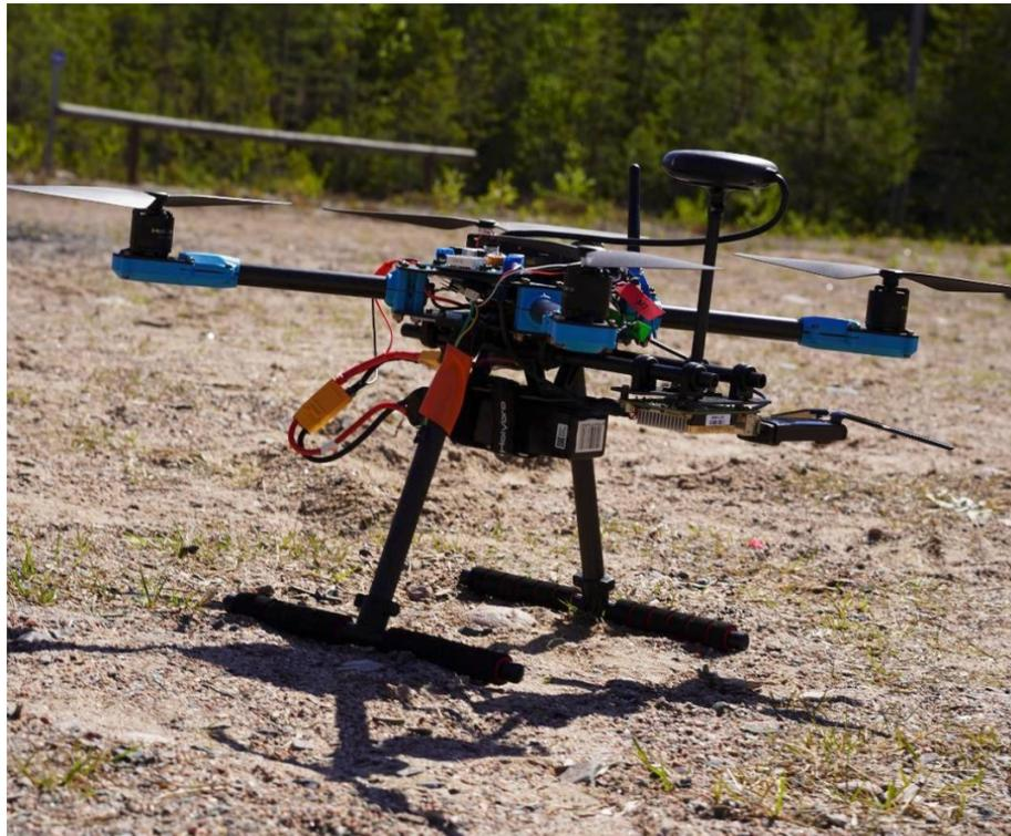
Figure 4.1: Holybro X500 V2 quadcopter equipped with onboard computer
