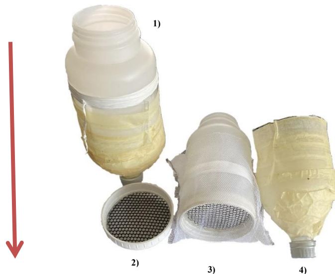
Figure 1 The new collector: 1) The whole collector covered with masking tape to protect from the sun, 2) the middle sieve (3x3mm), 3) the top part with the middle sieve and net mesh connected, 4) bottom part showing the bottle cap used as a valve. Arrow: shows the direction that insects sink in the collector.
