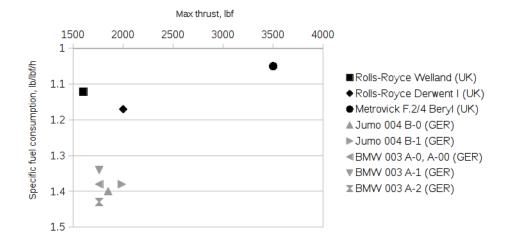
Figure 6: Performance and fuel efficiency of Second World War-era jet engines. Performance (maximum static thrust) increases towards top right. Data from Wilkinson (1946) and Kay (2002).
