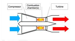
Figure 4: A schematic of a jet engine.
