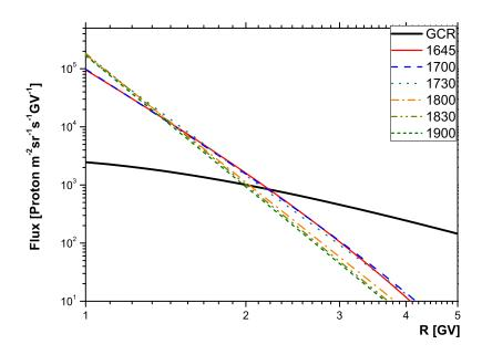
Figure 7: Derived SEP rigidity spectra during GLE 72 on 10 September 2017. The black solid line denotes the GCR particle flux, which corresponds to the time period of the GLE 72 occurrence and includes protons and  $\alpha$ -particles, the latter representative also for heavy nuclei. Time (UT) corresponds to the start of the five minute interval over which the data are integrated.
