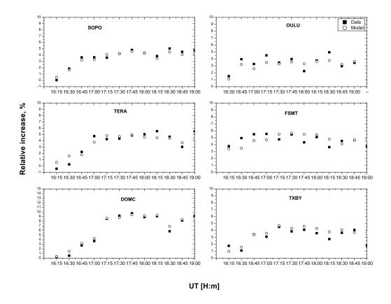
Figure 9: Modelled and observed responses of several NM stations during the GLE 72 on 10 September 2017. The accuracy of the fit for other stations is of the same order.
