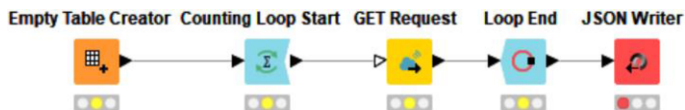
Figure 1. This workflow generates data of 10 patients based on the Template Pankreaskarzinom. From left, the first node creates an empty table. Second node starts the loop and numbers of loop can be set in the setting, in our case it was 10. Third node uses the link mentioned in text in step 3 and retrieve the data of a patient. Fourth node checks the conditions whether number of loops have been executed and collects the data. Once all the loops are executed, it ends the loop. Fifth node write the JSON files to given directory.
