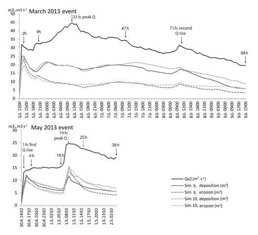
**Figure 5.** The hourly volumetric changes during the moderate- and low-magnitude flow events of March and May 2013. The results are based on simulations 9 and 10. The graphs show the erosion and deposition from the beginning of the flow events (12:00 on 5 March and 14:10 on 30 April) until the time when the erosion and deposition had declined and levelled out during the receding phases. The key time steps are pointed out as hours from the beginning of the flow events.
