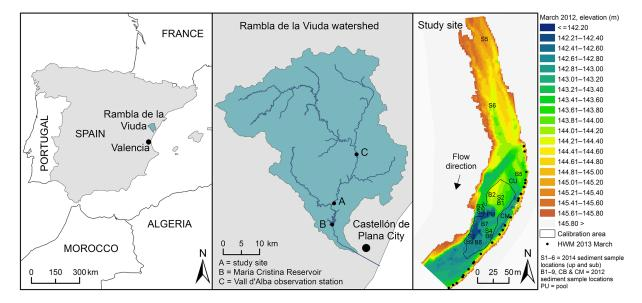
**Figure 1.** The study site of Rambla de la Viuda, eastern Spain. The elevation on March 2012 is derived mainly from mobile laser scanning data, but the edges are from the 2009 national digital elevation model. The calibration area was defined based on the data coverage of March 2013. The high-water mark (HWM) measurement locations of 2013 March are shown (their values are plotted in Fig. 3). Also, the sediment sample locations are shown (see also Table 2 and Fig. 2).
