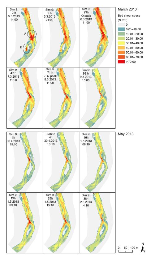
Figure 7. The bed shear stress of simulation 9 during moderate and small discharge events. The key time steps are presented (see Fig. 5).
