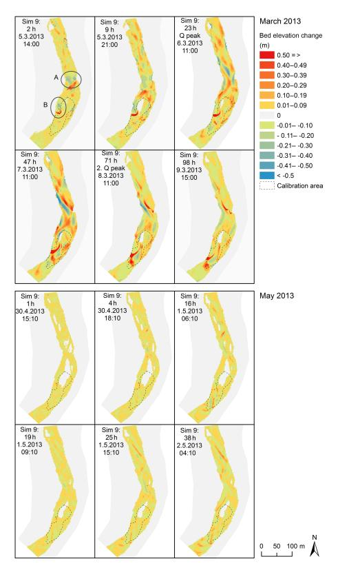
**Figure 6.** The modelled bed elevation changes between the key time steps of March and May 2013 events (see Fig. 5). The changes of the 5 March 2017 at 14:00 are from the beginning of the discharge event.
