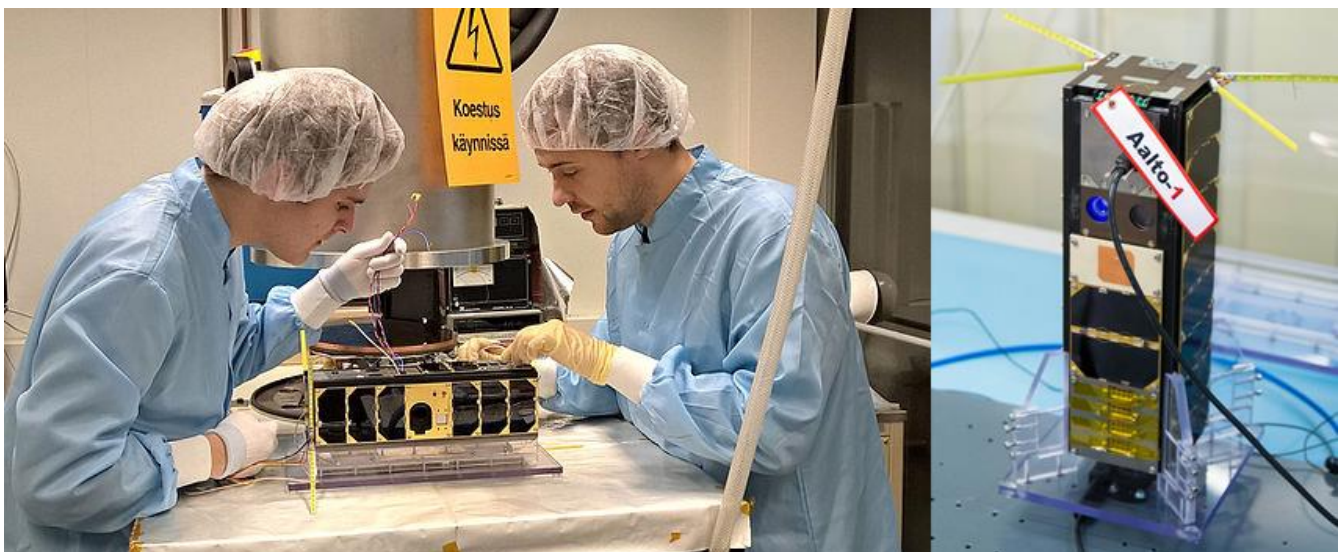
Figure 1. Aalto-1 quality manager Tuomas Tikka and systems engineer Antti Kestilä preparing the Aalto-1 satellite for thermal-vacuum test. The satellite Flight Model on the right.
