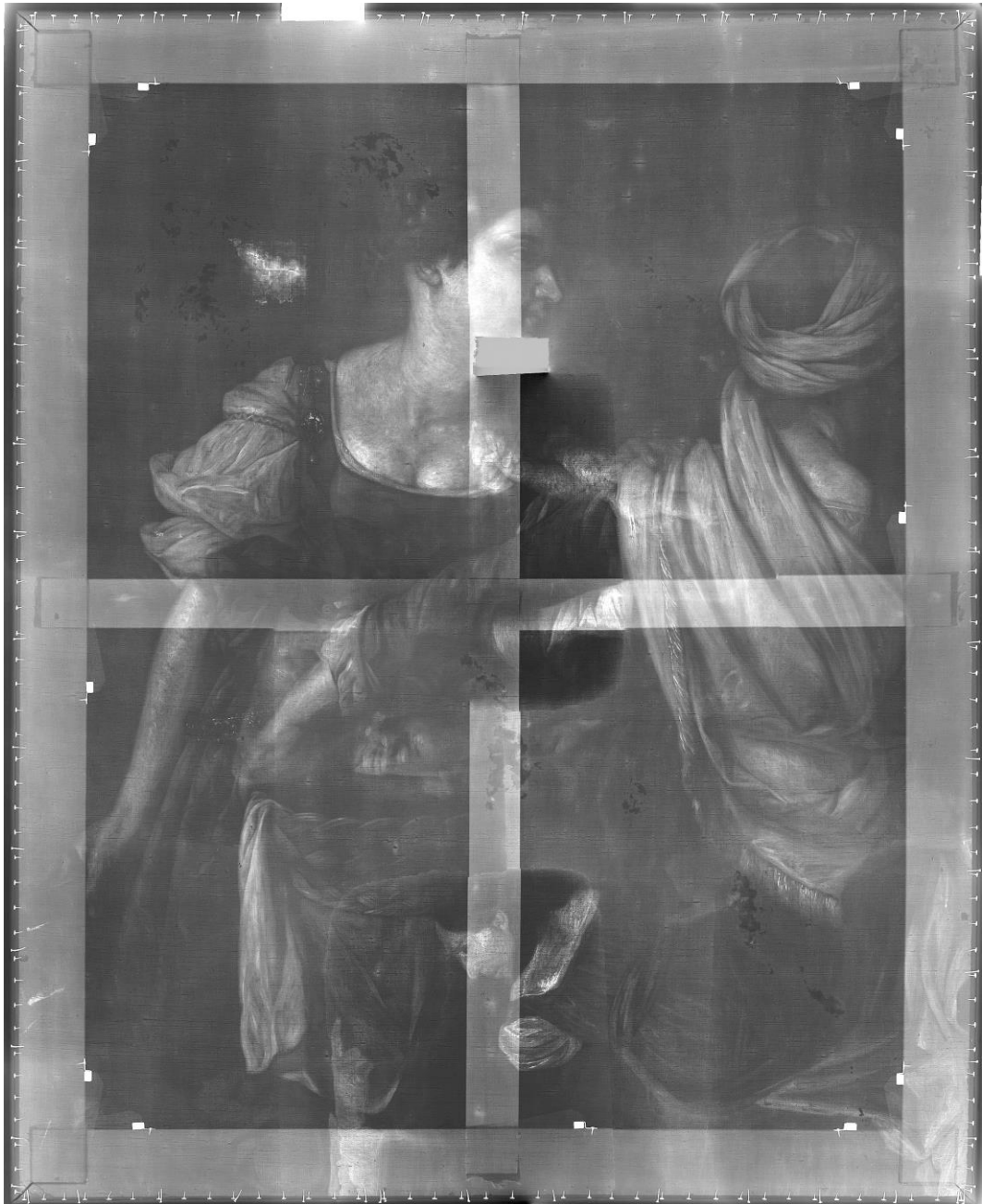
Figure 6. X-radiography image compilation showing another composition under Judith and Her Maidservant in the lower edge of the painting and also in the upper half situated between the shoulder lines of Judith and Abra. Metallic wedge or key holders and nails are visible around the painting as white areas. X-radiography images by Heikki Häyhä, digitally compiled by Emilia Laaksovirta.
