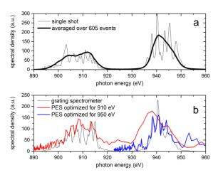
Figure 7: Experimental demonstration of two-color lasing: (a) single shot (thin line) and averaged over 605 events (thick line) spectral distribution measured with grating spectrometer; (b) single shot spectra measured with grating spectrometer (black line), with PES optimized for 910 eV (red line) and with PES optimized for 950 eV (blue line).
