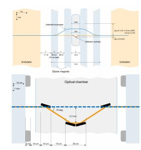
Figure 3: Concept of chicane and optical delay line.
