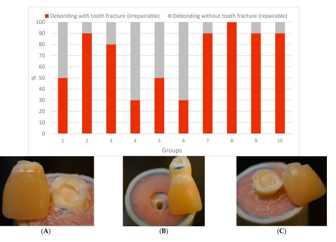
**Figure 4.** Percentages and photographs of failure modes of the tested restorations. (**A**,**B**) irrepairable fracture type, (**C**) repairable fracture type.
