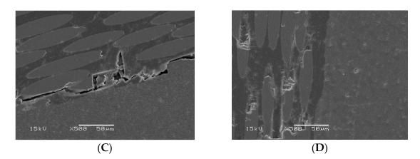
**Figure 5.** SEM images ( $\times$ 500 and 1000 magnification) of the adhesive interface (arrows) between fiber post and luting materials. (**A**) fiber post with Gradia Core before loading test, (**B**) fiber post with SFRC before loading test, (**C**) fiber post with Gradia Core after loading test (cracked), (**D**) fiber post with SFRC after loading test.
