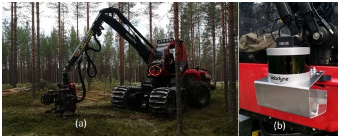
Figure 2. (a) Komatsu Forest 931.1 forest harvester. The LiDAR scanner is attached in the front of the windshield of the cabin (orange circle), giving a 210° view forwards. (b) A close-up of the LiDAR scanner.
