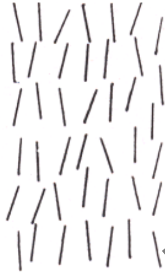
Figure 1. Schematic representation of molecules in nematic state.
