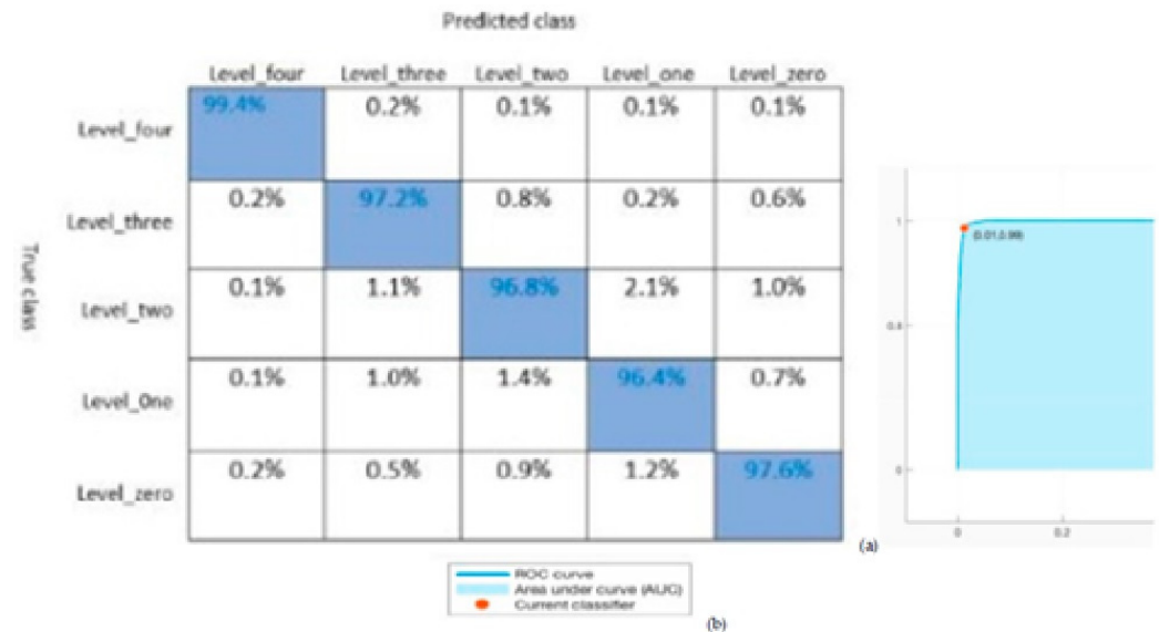
Figure 9. (a) The confusion Matrixes for the coarse K -NN classifiers given the accuracy for each class via a 5-fold cross-validation of 99.4%. (b) The ROC curve figures generated from the Medium K -NN classifier. The dark blue line is the ‘ROC curve’; the light blue region is the ‘Area under the curve’; and the red dot is ‘Current classifiers’.
