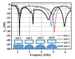
Fig. 2. The S-parameters of the four antennas.
