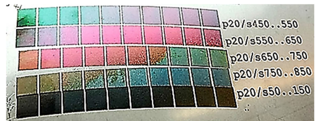
FIGURE 4. The dependency of produced color on the scanning speed ( I_0 = 1.6 \cdot 10^8\ \text{W/cm}^2 , f = 60\ \text{kHz} , \tau = 100\ \text{ns} , H = 0.01\ \text{mm} , V_{sc} = 450\text{-}850\ \text{mm/s} : line 1 to 4 and V_{sc} = 50\text{-}150\ \text{mm/s} : line 5 from left to right).
