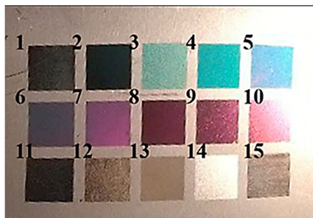
FIGURE 17. Color palette after 24hr of exposure in the environmental test chamber at temperature - 40 °C and humidity 90%.
