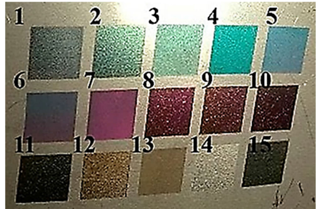
FIGURE 19. Color palette after 24hr exposure in the environmental test chamber at temperature 40\ ^\circ\text{C} and humidity 70%.
