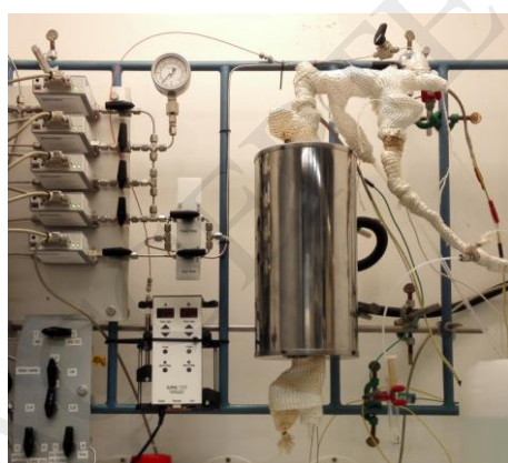
Figure 1. Schematic presentation of the fixed bed reactor for catalyst evaluation.
