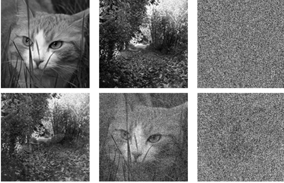
Fig. 2. The first row shows the original signal images plus one exemplary noise component from \mathbf{Z} . The second row shows the first three estimated components \hat{\mathbf{Z}} when using FOBI. All components not shown look like the noise components (third column).
