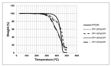
Fig. 1. TGA of 20 to 50 wt.% OPF reinforced PP composite materials
