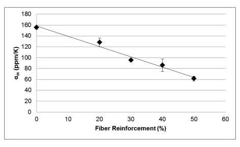
Fig. 5. Coefficient of thermal expansion as a function of fiber content
