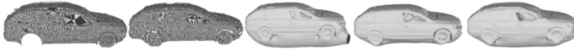
Figure 12. Car reconstruction from different point densities by the methods of the Crust and SPR. Left two images: the Crust with the resampling points of 0.01 m and 0.05 m, respectively; Right three images: the SPR with the original points and the resampling points of 0.01 m and 0.05 m, respectively.
