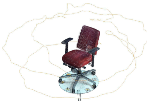
Figure 5. An object point cloud reconstructed with a hand-held scanner shown with the measurement trajectory and automatically detected markers mounted adjacent to the object on the table surface.
