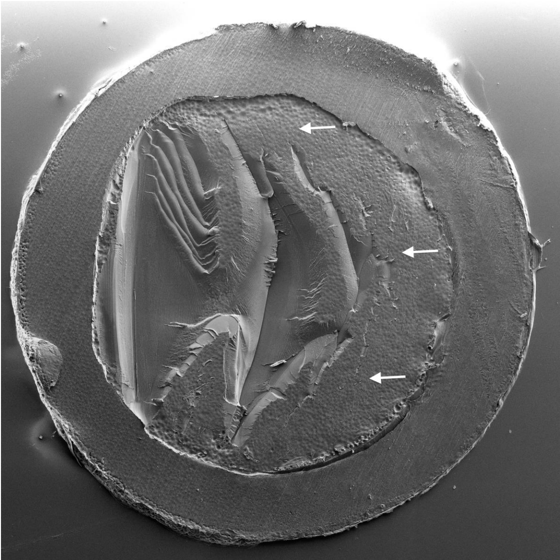
Figure 2. Scanning electron microscopy (SEM) image of the partially adhesive type failure observed in the vacuum mouldable thermoplastic plates after SBS test. Key: arrows show the areas with adhesive failure.
