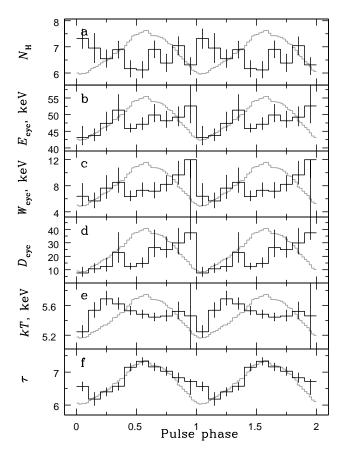
**Figure 5.** Dependence of the spectral parameters of XTEJ1858+034 on the pulse phase revealed from the *NuS-TAR* data. Different panels correspond to the absorption column in units of  $10^{22}$  cm<sup>-2</sup> (a), cyclotron line energy (b), width (c) and strength (d), comptonizing plasma temperature (e) and optical depth (f). Pulse profile in 3-79 keV energy band is shown in grey for clarity.
