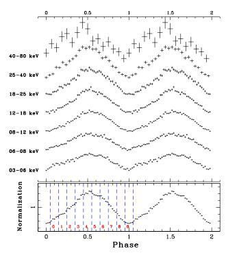
**Figure 2.** *Top:* Pulse profiles of XTE J1858+034 obtained with *NuSTAR* in different energy bands. The profiles are shown twice in phase and arbitrarily rescaled in count rate for clarity. *Bottom:* Pulse profile of XTE J1858+034 in the full energy band 3–79 keV with phase bins selected for the phase-resolved spectral analysis shown with vertical dashed lines.
