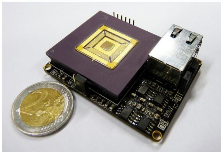
Fig. 3. KOVA1 embedded camera module by Kovilta, an industrial partner in MARIN project.
