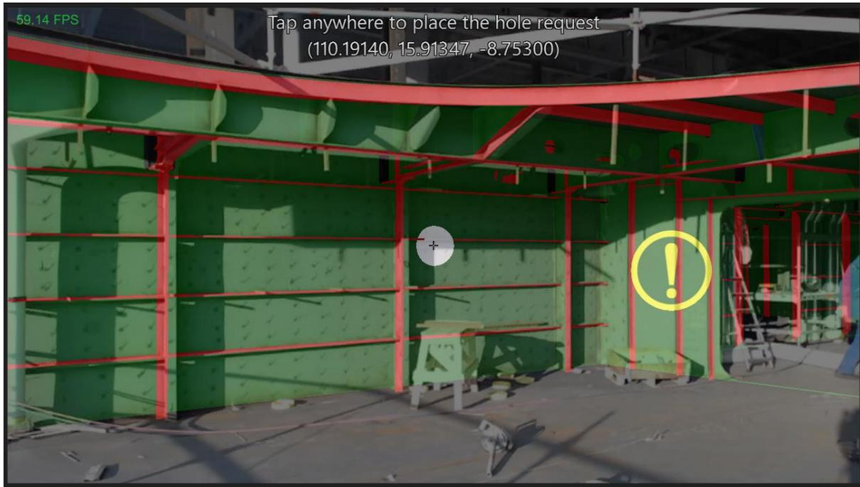
Fig. 6. Opening request application prototype screen. User sees the 3D model superimposed on real environment. The blob with a + sign is a virtual sphere used as a pointer for placing the opening onto a surface.
