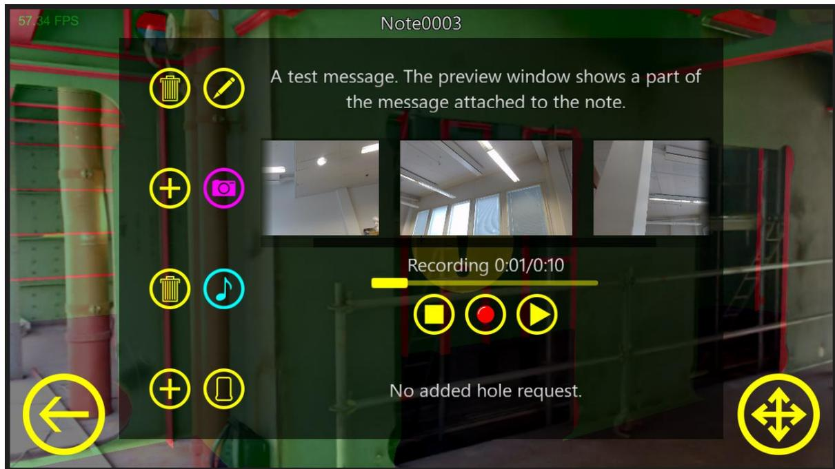
Fig. 5. Documentation application prototype. Text, photos and audio messages can be included in a note that is placed virtually in a location in the ship.
