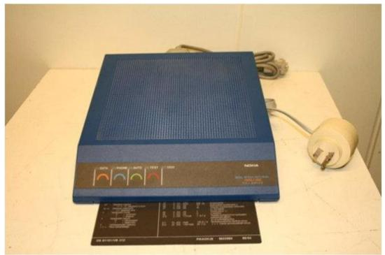
Picture 1. Nokia started to manufacture modems in the late 1980s. In the picture, VB 312 -modem from 1987, which supported dual speed mode (300 b/s and 1200 b/s). VB 312 was advertised with a slogan "For hackers and other professionals". (MikroBitti 4/1987). Source: Salo Museum of Electronics.
