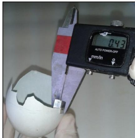
Figure 6. Measurement of eggshell thickness at equator (Photo: Toxicology and Forensic Veterinary Medicine group, University of Murcia, Spain. http://www.sertoxmur.com/ ).
