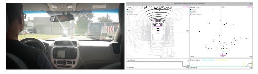
**Figure 7.** Snapshot of testing use-case with a pedestrian crossing the road without paying attention. Image on the right shows GUI (colours inverted) for the Aurix-based processing of LIDAR and RADAR data, heartbeat monitoring and break actuation.
