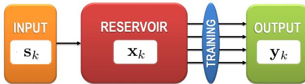
Figure 1: The basic structure for RC is formed by an input layer, a reservoir, and an output layer. The information contained in the input is introduced to the reservoir, whose internal connections act as a fixed hidden layer. Some of the responses of the reservoir are used to produce the desired output after an optimization procedure during the training process (only the output connections are adapted in the training).
