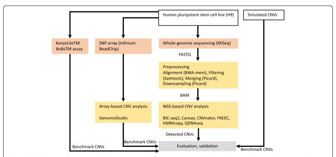
**Fig. 1** Flowchart showing the main steps of our comparison, including preprocessing of the data, detection of copy number variations (CNVs) with six different algorithms (BIC-seq2, Canvas, CNVnator, FREEC, HMMcopy, and QDNAseq) and evaluation and validation of the results. The karyotyping results from the KaryoLiteTM BoBsTM assay are from an earlier study [9]
