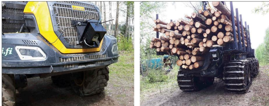
**Figure 2.** The 2D Light Detection and Ranging (LiDAR) sensor mounted on the rear of the Ponsse Scorpion King harvester (left) and on the Ponsse Elk forwarder (right).
