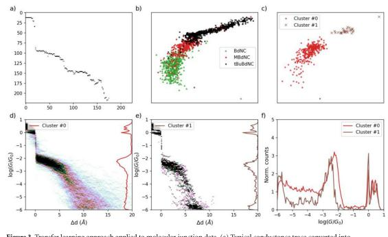
**Figure 3.** Transfer learning approach applied to molecular junction data. (a) Typical conductance trace converted into  $224 \times 224$  b/w image. (b) AlexNet-based dimensionality reduction approach applied to the molecular junction data for three molecules. (c) Two clusters for MBdNC molecule, determined by the Spectral Clustering algorithm.( d-e) Combined 2D/1D conductance histograms for clusters 0 and 1, respectively. (f) Conductance histograms for clusters 0 and 1.
