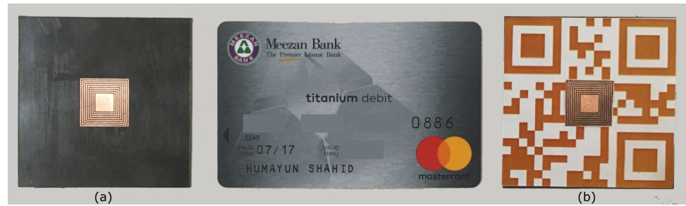
Fig. 3. (a) Electromagnetic data encoding circuit. (b) QR-incorporated chipless tag.
