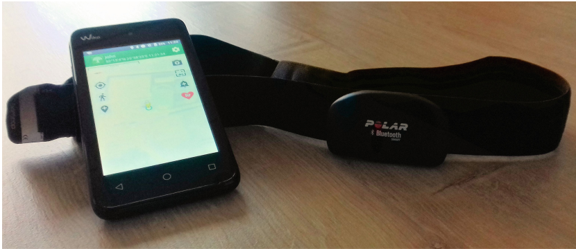
Fig. 4. A smartphone with SGN application running together with Polar H7 heart rate sensor.
