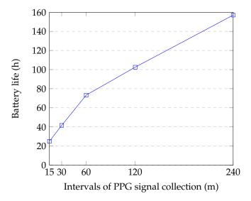
**Figure 9.** Battery life time of the watch for different intervals. Each interval contains 12 min of PPG signal collection.
