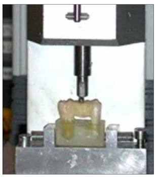
Figure 3. Placement of the steel ball to occlusal fossa.
