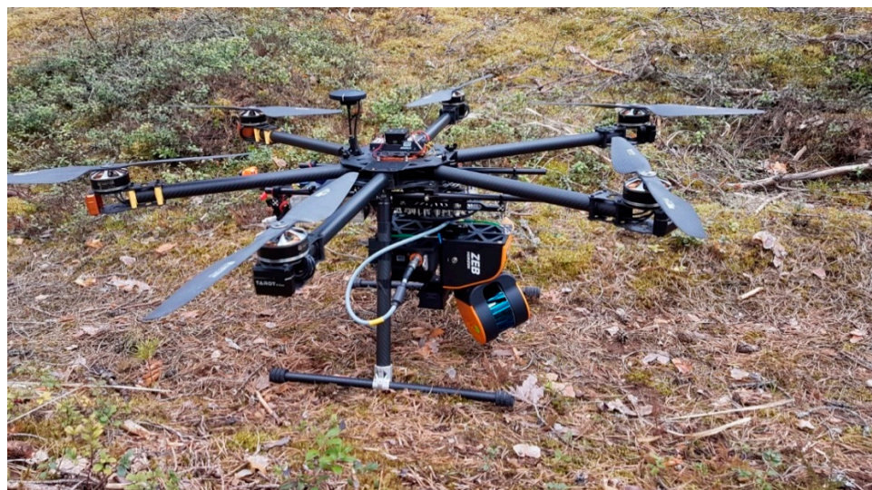
Figure 2. UAV equipped with a rotating laser scanner developed for the study.
