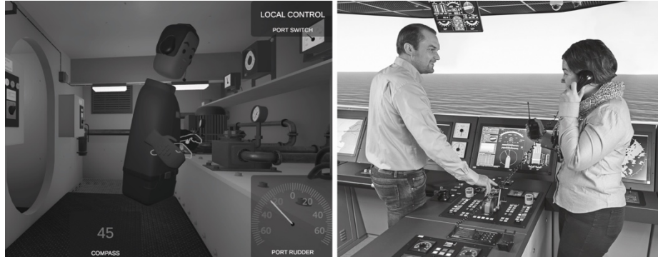
Fig. 2. The instructor view in the Steering Gear room VR-simulation (Left) and decision making and communication in a bridge simulation exercise (Right).
