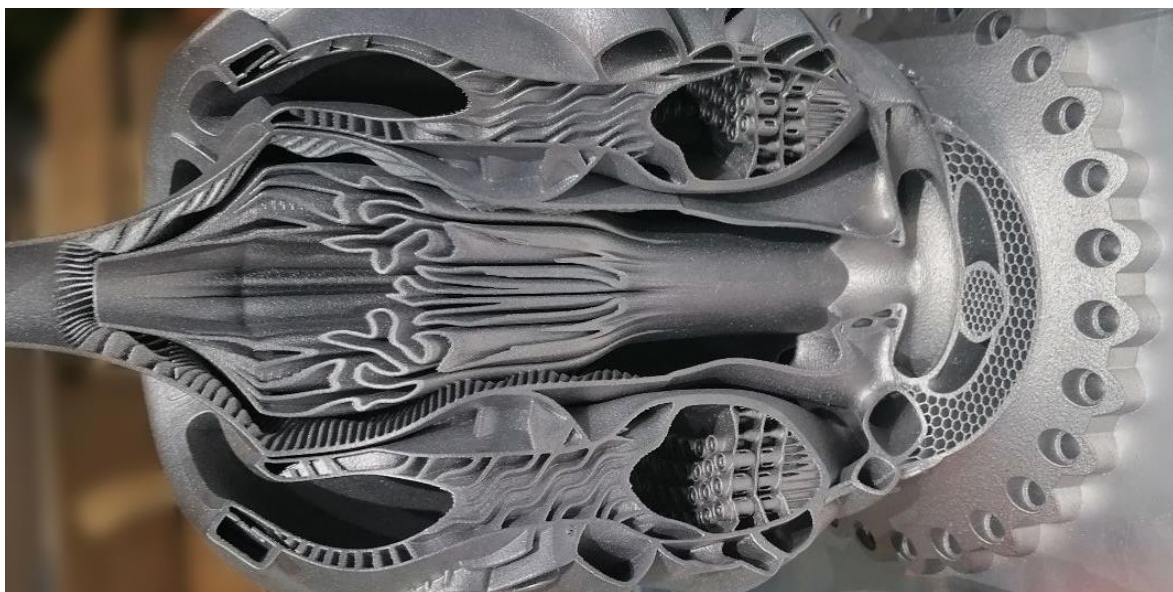
Figure 12: A cross-section of a rocket engine optimized by artificial intelligence. Picture: Patricia Nyamekye. The object was designed using algorithms by Hyperganic and manufactured by EOS.
