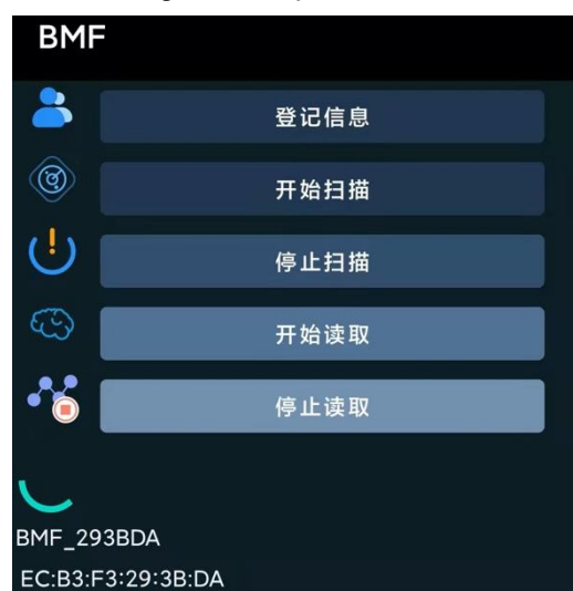
Figure 5-4 The interface between the mobile phone and EEG acquisition device (From top to bottom, the buttons are for subject's information registration, start scanning, stop scanning, start loading data and stop loading data)
