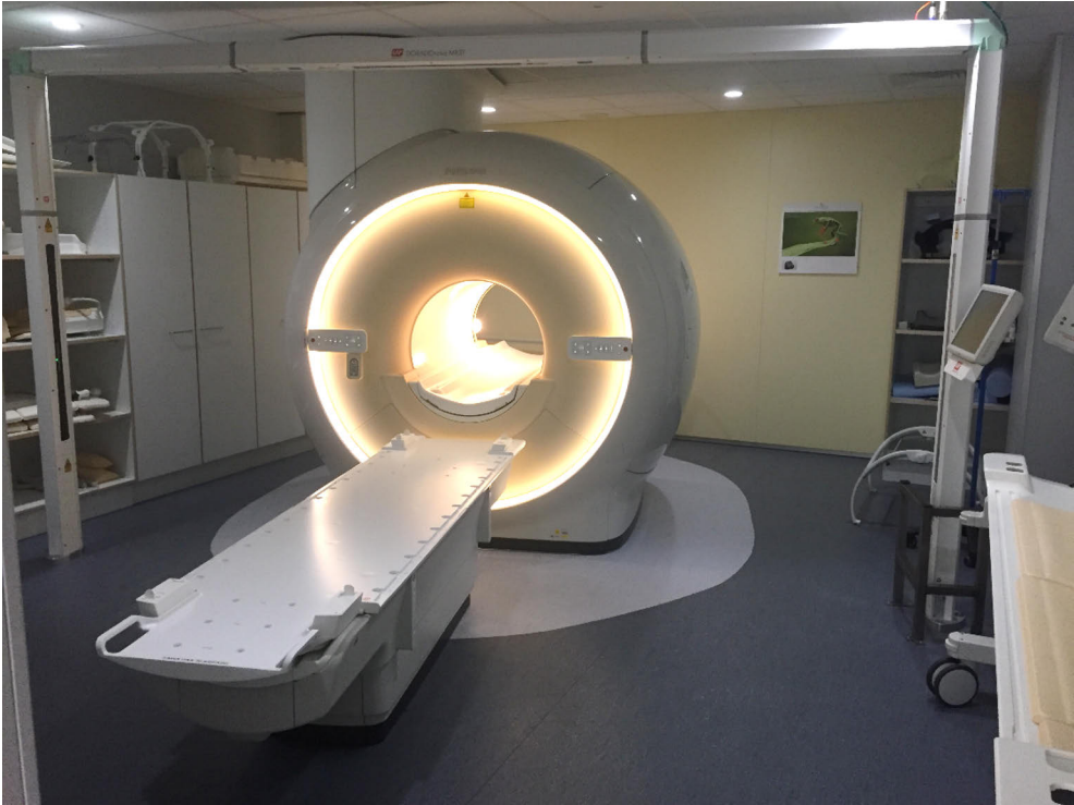
Figure 1. Philips Ingenia 1.5 T MR-RT magnetic resonance imaging (MRI) system and the LAP DORADOnova MR3T external laser positioning system (ELPS) located at the Department of Oncology and Radiotherapy of Turku University Hospital (Tyks, Turku, Finland).
