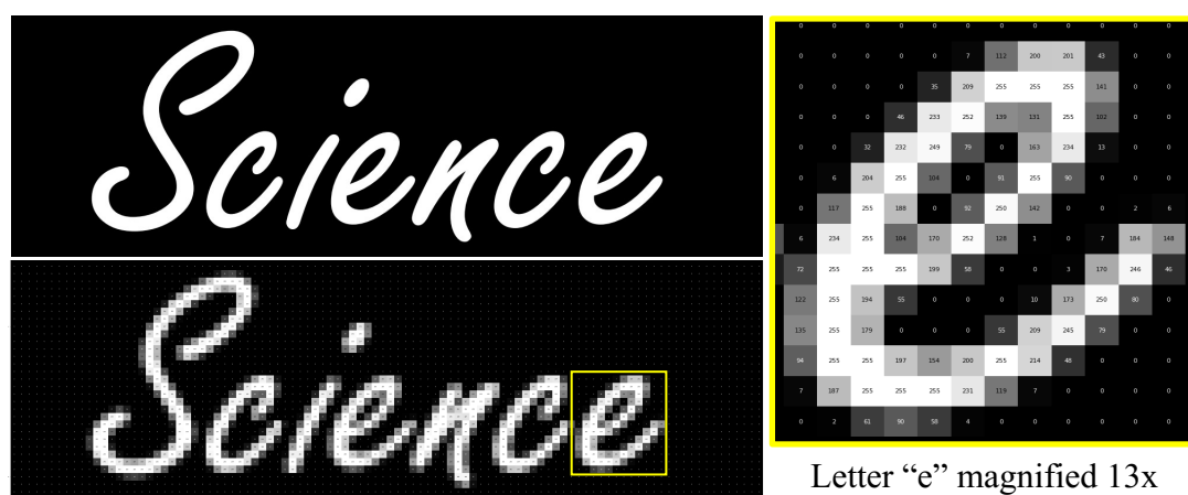
Figure 3.1: Top-left is the mode by which a digital device illustrates an image. Top-bottom map's pixel brightness intensities. The highlighted yellow area shows the relationship between pixel value and brightness intensity.
