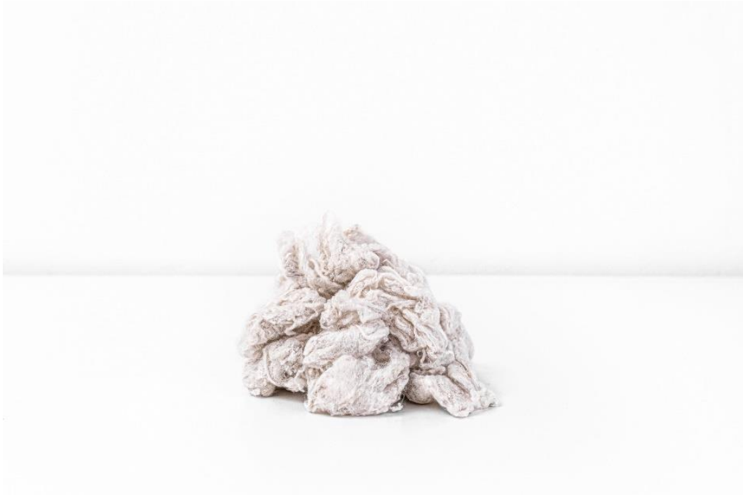
Figure 6: Regenerated Infinna™ fibre from textile waste. Picture by Daily Mail (2020)
