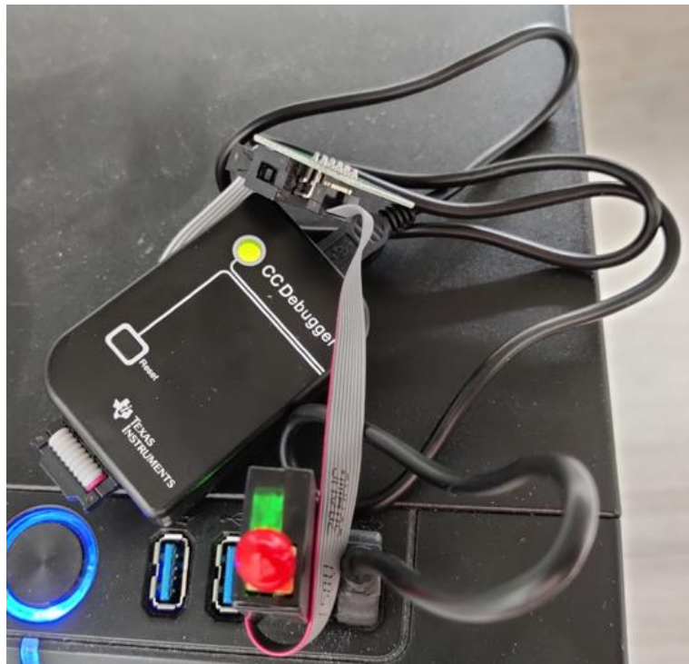
Figure 6. Connecting the CC debugger and USB dongle to a Windows 10 desktop computer (CC debugger light is green).
