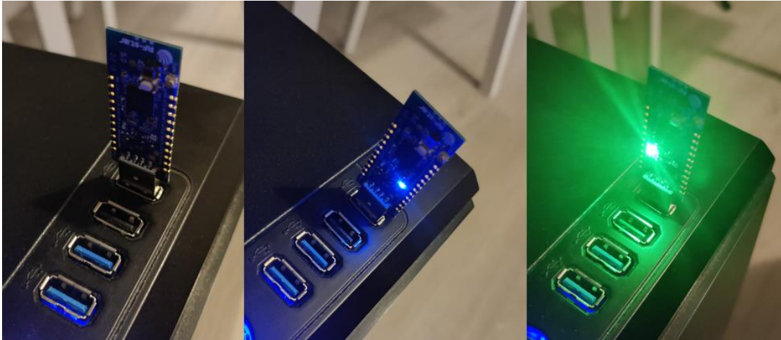
Figure 20. Inserting the nRF 52840 dongle to Windows 10 machine (no light), pressing the reset button on the USB dongle (blue flashing light), flashing the USB dongle with the sniffer firmware (green flashing light).
