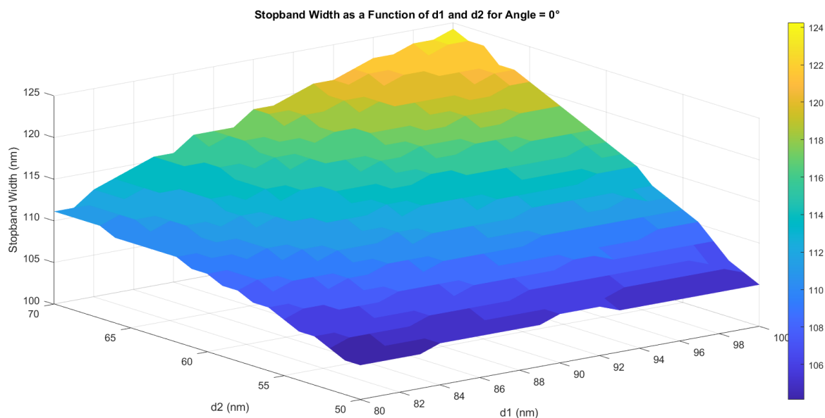
Figure 10: Stopband width of a DBR as a function of layer thicknesses.
