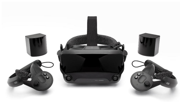
Figure 5. The Valve Index VR headset, its Knuckles-controllers, and base stations [40].
