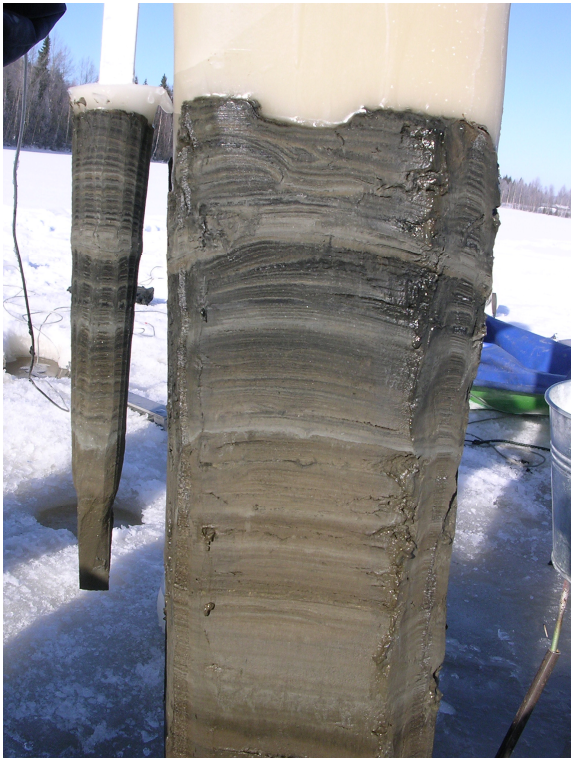
Figure 2. Freeze cores taken from Kortejärvi in March 2004 with two types of ice fingers. The length of the “mini ice finger” on the left is ca. 20 cm. Note the undisturbed water-sediment interface (Photo courtesy of T. Saarinen)
