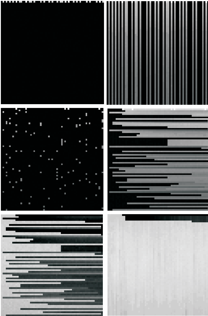
Figure 8.20: Measurements from the MIPA4k CNN processor configured in gray scale mode of operation, corresponding to Figures 8.16, 8.17, and 8.18. For technical reasons, the first four computing steps are performed on inverted values of Boolean variables, and the cell states are then inverted in the fifth step.
